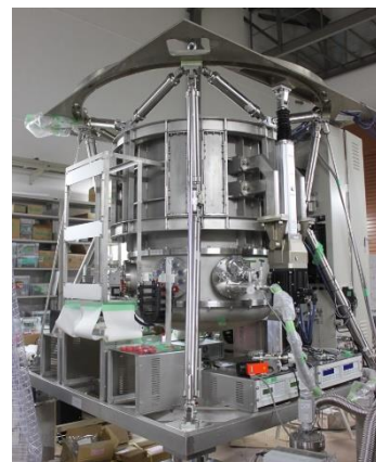
MIMIZUKU at Mitaka Lab. Dimensions are 2.0 \times 2.0 \times 2.1 m 3 . Weight is 2.5 tons.
