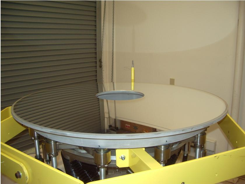
M2a Secondary Mirror after flexure bonding, being prepared for lift into enclosure
