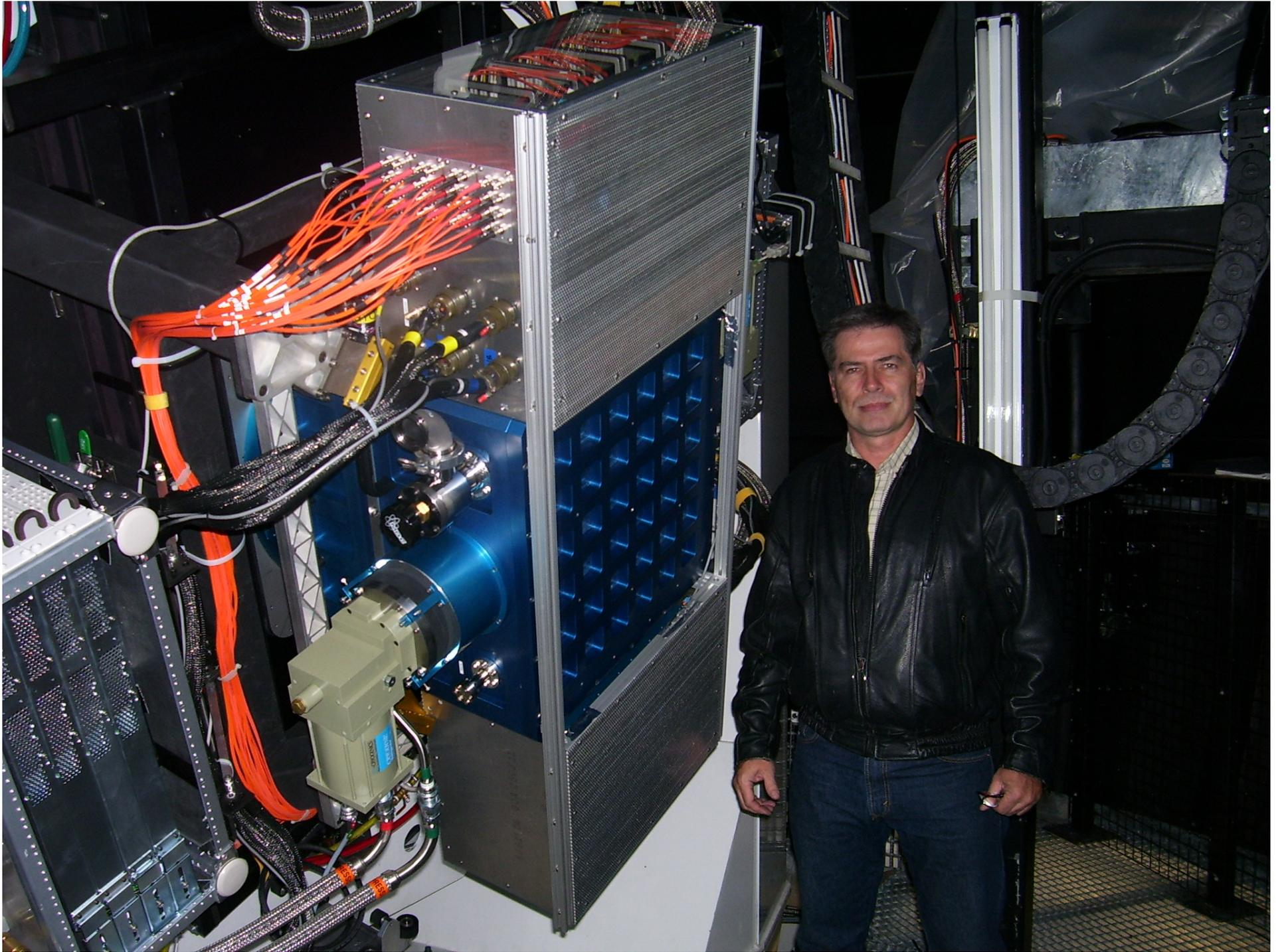
PS1 Calibration Unit – back illuminated screen with projector fiber fed from NIST tunable laser - Measure the system throughput as a function of wavelength for every pixel every day.
