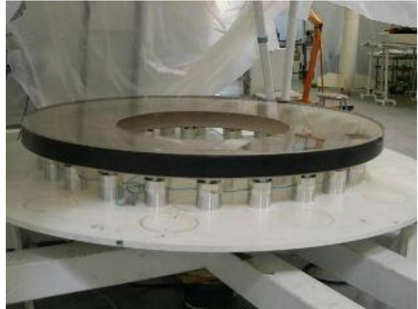
M1 Primary Mirror with protected aluminum coating prior to lift into enclosure
