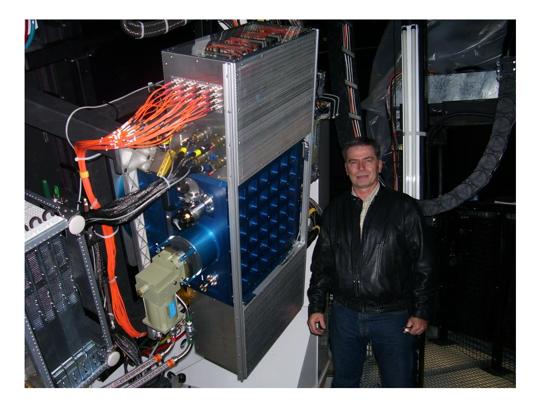
PS1 Calibration Unit – back illuminated screen with projector fiber fed from NIST tunable laser - Measure the system throughtput as a function of wavelength for every pixel every day.
