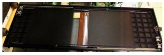
Carbon fiber construction 40 cm aperture Blade trajectory repeatable to 10 millisec! Timing interface with GPS University of Bonn
