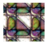
Orthogonal Transfer Array: A new pixel/CCD chip design to noiselessly remove image motion at high speed (~10 usec)
