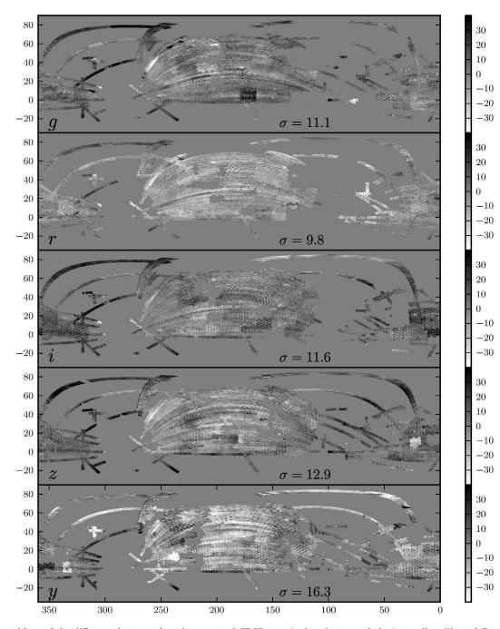
FIG. 5.— Maps of the difference between the color-corrected SDSS magnitudes of stars and the internally-calibrated Pan-STARRS1 magnitudes of the same stars in the filters  $grizy_{P1}$  (rows). The x-axes give right ascension and the y-axes give declination. The rms of the maps is about 10 mmag. Narrow stripes in right ascension are symptomatic of problems with the SDSS photometric calibration, while rectangles in right ascension and declination indicate problems with the PS1 calibration.
