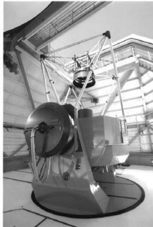
left : an equatorial mount telescope, the English yoke of the 3.8 m U.K. Infrared Telescope (UKIRT)
