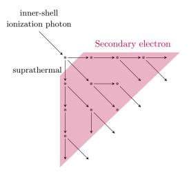
Neutral atoms are ionized and secondary suprathermal electrons are produced one after another.
