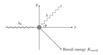
Compton effect : a process in which photons are scattered by an electron. Its cross section is known as the Thomson electron-scattering cross section  $\sigma_{\rm T} = 0.66 \times 10^{-24} {\rm cm}^{-2}$ .
