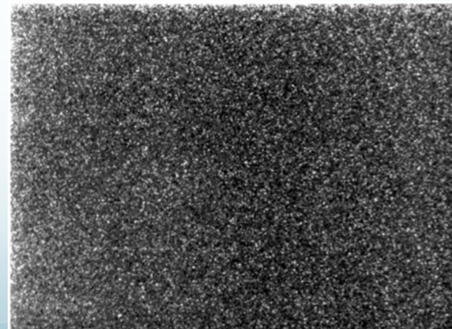
Figure 9.6. A clean bias frame showing no serious amplifier fixed pattern noise or faint diagonal bars due to ground-loop interference.
