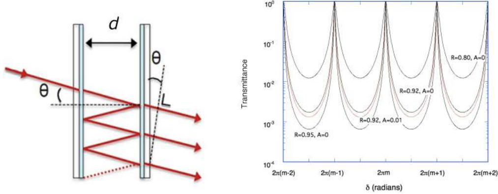
Figure 1. (left) Principle of Fabry-Perot interferometry. (right) Transmittance profile of Fabry-Perot interferometer (Airy function).
