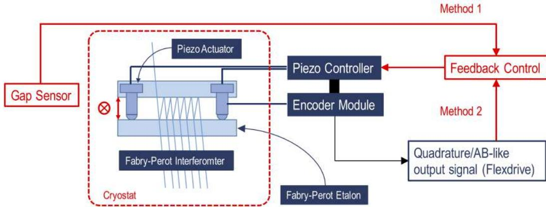
Figure 2. Conceptual design of tunable Fabry-Perot interferometer control system.
