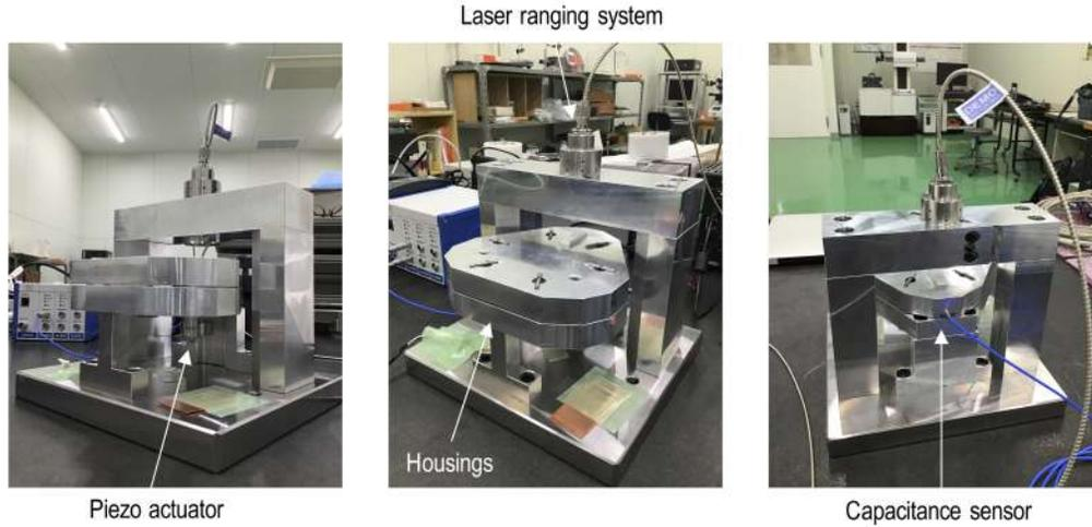
Figure 6. Measurement setup (1 axis).
