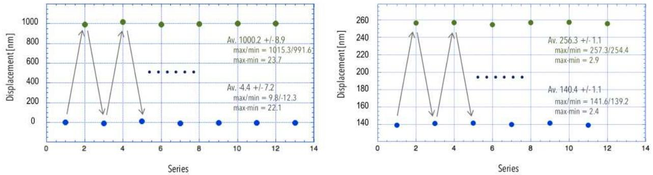
Figure 7. Results of multiple repetitive test (left : long range, right : short range). Uncertainty (stdv) before and after movement are about (1) 10 nm and (2) 1 nm respectively. Time drift was corrected for each results.
