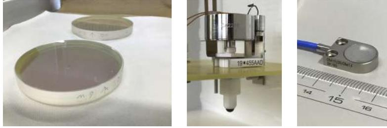
Figure 4. (left) Etalon (center) Piezo actuator (right) Capacitance gap sensor.
