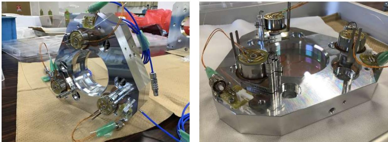
Figure 5. Aluminum housing with each component mounted.
