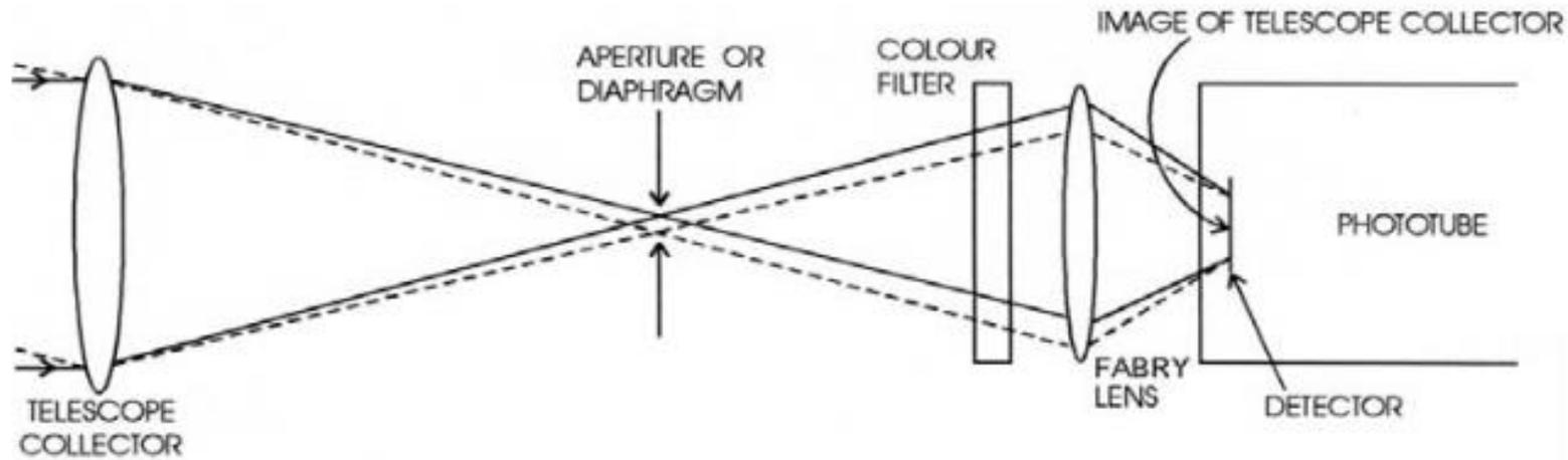
Light from the star remains stable on the detector even if the star drifts within the aperture. Light from the star is focused through the aperture, filter, and Fabry lens onto the PMT, producing a stable signal.
