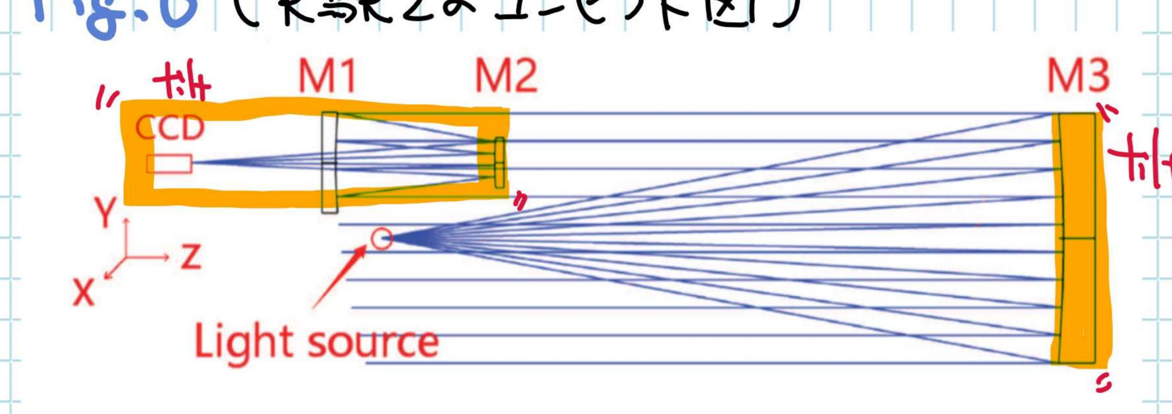
Figure 6. The concept design of the optical path in our experiment.
