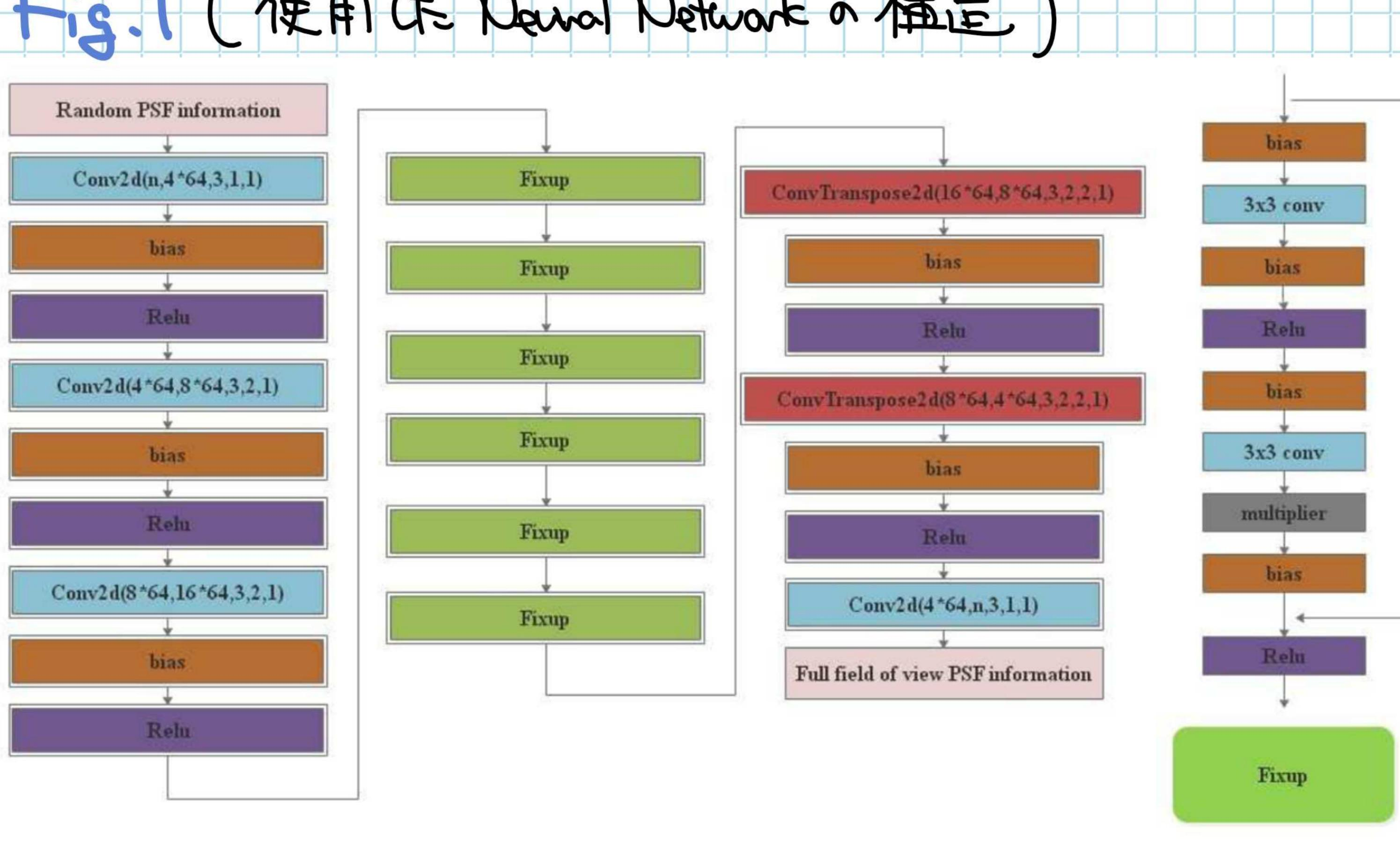
Figure 1. The structure of the Tel-Net. The Tel-Net consists of convolutional layers (Conv2d in blue), Bias layers (Bias in brown), Activation layers (Relu in purple), Conv-transpose layers (ConvTranspose2d in red), multiply layers (multiplier in grey) and Fixup blocks (Fixup block in green). The structure of Fixup block is shown in the right part of this figure.
